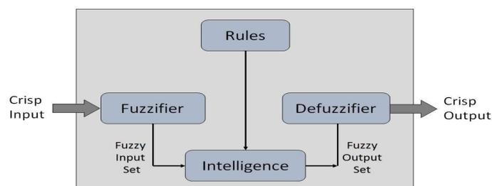
Fig 8: The above flowcharts shows the Fuzzy Logic Controller
