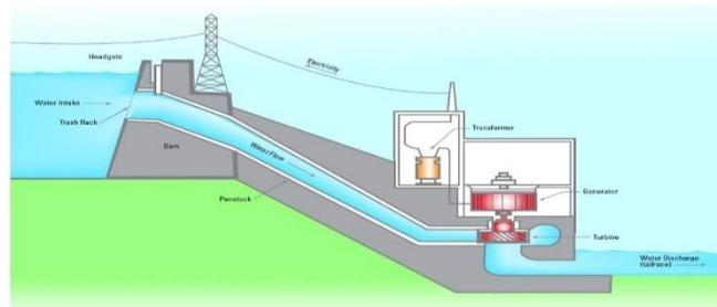
Fig 3: The figure shows the layout of Hydro Power Plant Structure
